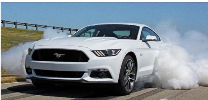
of a drag strip, the driver can apply the accelerator to spin up the rear wheels to warm the tires for maximum grip. This can all be done without having to balance one foot on the brake and the other on the gas, or install a mechanical line-lock.
