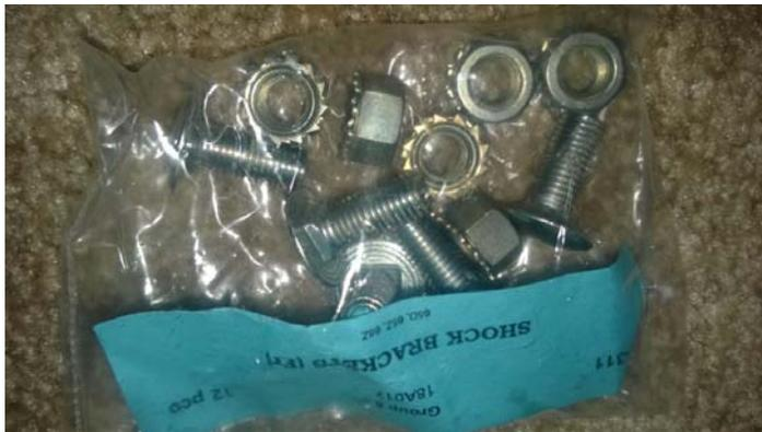
These are the nuts and copper sealing washers used on the differential 3<sup>rd</sup> member.
