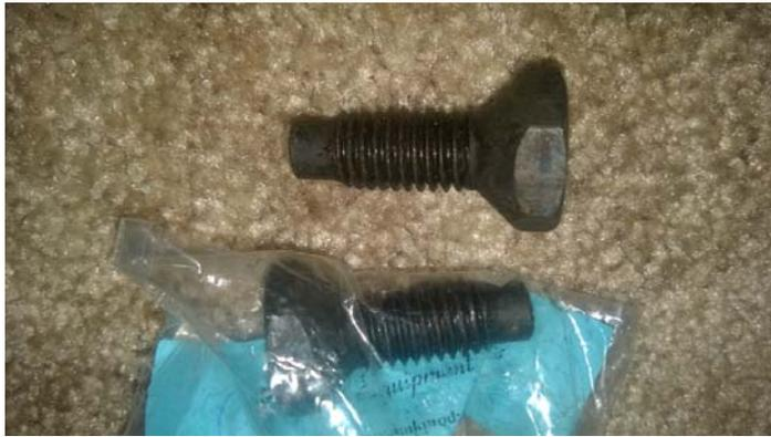
These are the Front Shock upper mounting bracket bolts. At first look, they appear to be carriage bolts. These are unique in that the heads are much slimmer (thinner) than a standard carriage bolt and those for '65 & '66 are fine thread, not coarse like later years.
