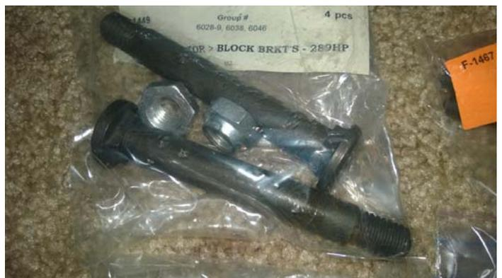
Bolts for the Ford Front Support Brace under the Engine, shown at the top of the next page, are also totally unique. Because of their location, these guys particularly like to rust into the frame.
