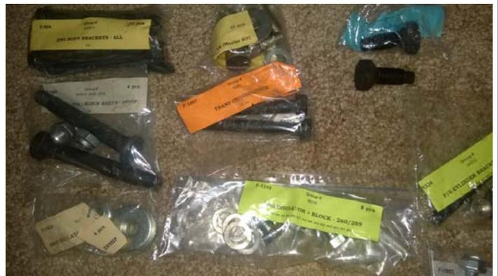
In another example, pictured here are the Motor Mount bolts. The bolt heads are totally unique, and the low profile nuts are not a common hardware store part.
