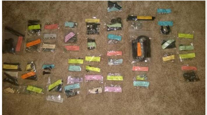
The kits are application specific to year, body, engine, and brake system type. Each of the colored tags are groups of fasteners, very specific to the area of installation.
